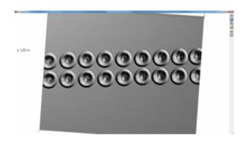
Typical tasks in quality assurance and research are the characterization of surfaces with different roughness (wafer structures, mirrors, glass, metals), the determination of step heights and the precise measurement of curved surfaces such as microlenses. The efficient, robust and highly accurate evaluation algorithms contained in the software are the result of extensive research.
