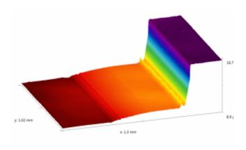
The measurements are based on the interferometric method. This is based on the fact that spatial and temporal coherent light wafes can overlap. The beams of the illumination device are divided by a beam splitter. One part of the light reaches the object surface, the other part generates a reflection by reaching a reference mirror. Due to the parallel acquisition and processing of the measuring points, height information can be obtained over a large area and in a very short time.
