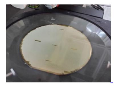
Vakuum Chucks with a finest porous surface for sawn wafers on blue tape. Even wafers with minute dies are sucked in safe and even.
