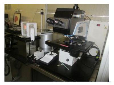
Inspection of masks used to produce wafers.
