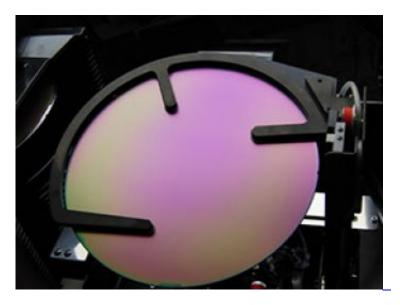
Bonded wafers are considerably thicker than single wafers and can have an offset. They may be noncircular. To solve various measurement and inspection tasks, Promicron relies on a large number of optical methods. They are combined according to requirements and customer request.
